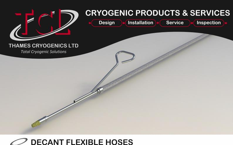
Decant Flexible Hoses are a special variant of our non vacuum insulated hoses made specifically for the purpose of decanting liquid nitrogen from a pressurised dewar or SIVL into an open vessel. The hoses are typically 1 - 2m in length and come fitted with a rigid tube, sinter and handle. The sinter is designed to give a good gas-free stream of liquid into the vessel and is protected by a shroud to prevent damage.
